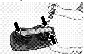
5. Remove the bulb strip from the tail light lens.
